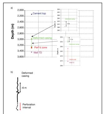
FIGURE 1: a) Relative vertical positions of casing deformation, cement return heights, perforation interval and well depth at well N42; b) Multiple doglegs formed at N42. Relative position and severity of the doglegs are based on the field data; but their absolute severity is for illustration purposes only.
