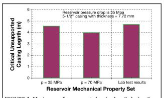
FIGURE 3: Maximum safe unsupported casing length during the well washing at N42. The x-axis denotes different sets of material properties whose details are listed in Table 1.
