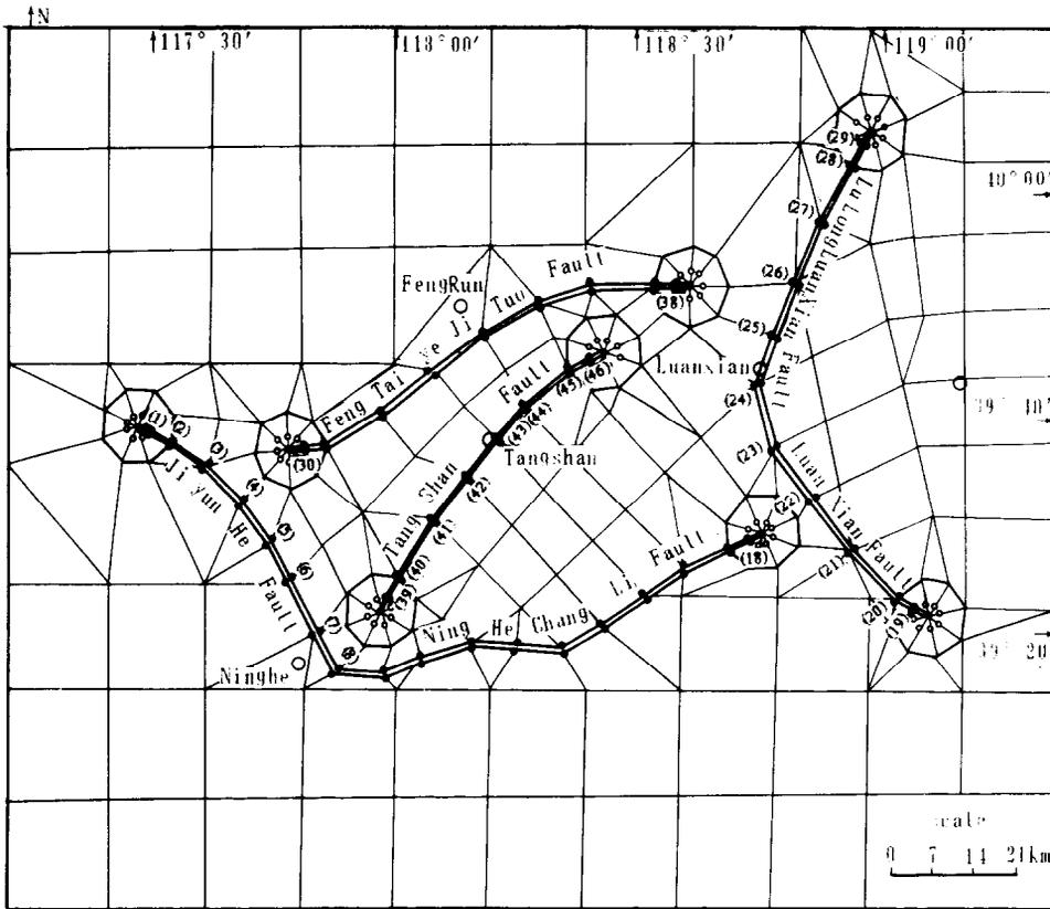
Fig. 1. Tectonic and finite element mesh map of the Tangshan rhombic block. The dots and circle form a series of nodal pairs along the surface to form a set of contact elements and the quarter-point node of the triangular elements, respectively. The numbers in parentheses indicate the sequence of nodal pairs.
