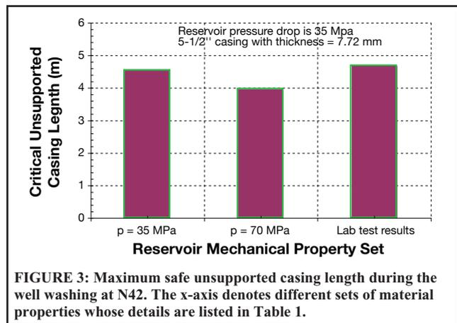
**FIGURE 3: Maximum safe unsupported casing length during the well washing at N42. The x-axis denotes different sets of material properties whose details are listed in Table 1.**
