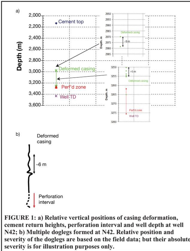
**FIGURE 1: a) Relative vertical positions of casing deformation, cement return heights, perforation interval and well depth at well N42; b) Multiple doglegs formed at N42. Relative position and severity of the doglegs are based on the field data; but their absolute severity is for illustration purposes only.**
