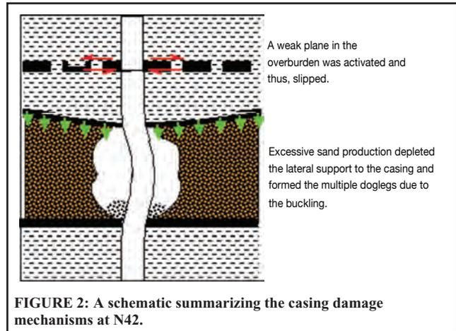
**FIGURE 2: A schematic summarizing the casing damage mechanisms at N42.**
